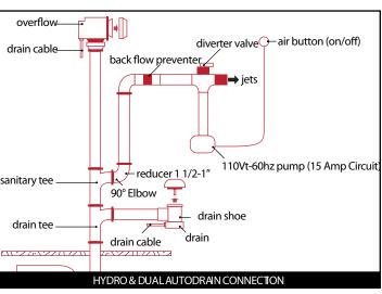
NOTE WE HAVE TAKEN RESPONSIBLE PRECAUTIONS TO ENSURE THE HIGH-SPEED AUTODRAIN IS SUITABLE FOR RESIDENTIAL PLUMBING. IT IS RESPONSIBILITY OF THE INSTALLER TO INSURE THE SANITARY SYSTEM IS ACCEPTABLE FOR THE USE OF THE HIGH-SPEED AUTODRAIN. WE DO NOT ACCEPT RESPONSIBILITY FOR DAMAGE ARISING FROM THE USE OF THE HIGH-SPEED AUTODRAIN.\*
